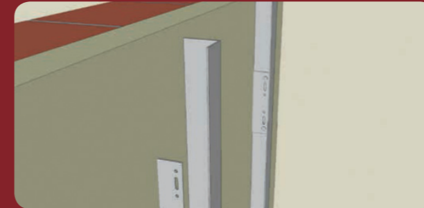
Installation of the first tile row with bottom clamps and fixing of joint profiles
