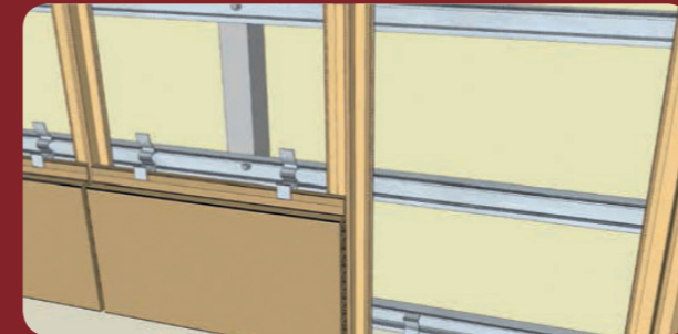
Installation of the top tile row
