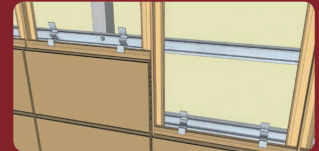
Installation of middle tile rows with middle clamps
