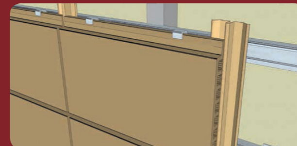
Installation of the top tile row
